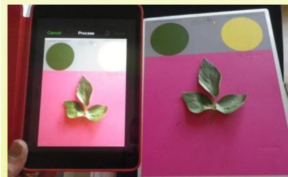
Figure 4. Using the FIELDSCOUT Greenindex to determine leaf colour.
