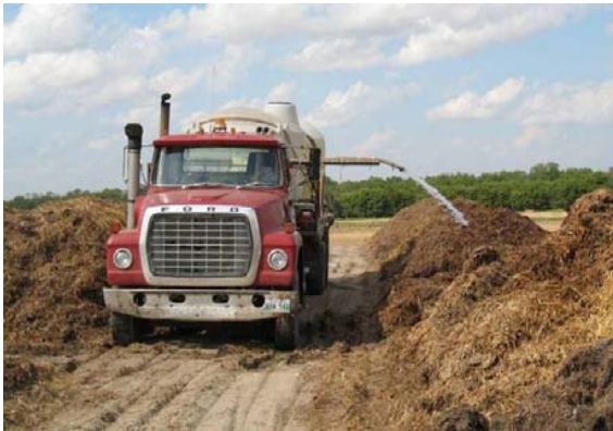
Water truck used to add moisture to the windrow
