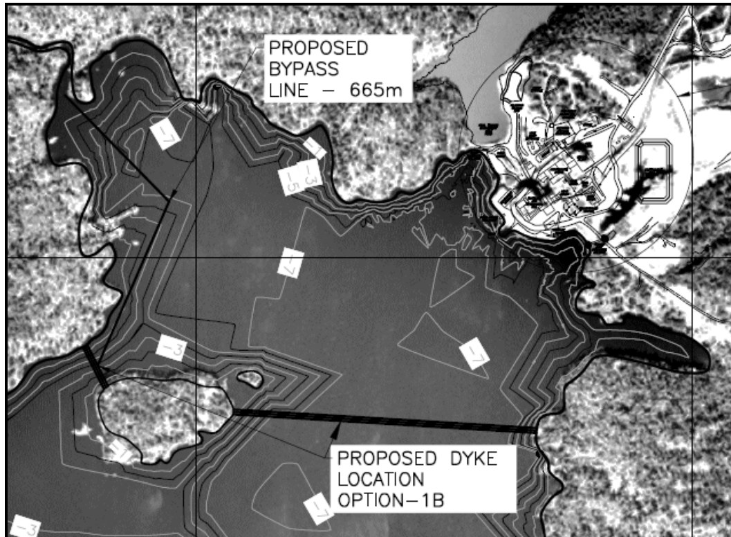
Figure 3.5 Option 1B, Dike Location Plan View
