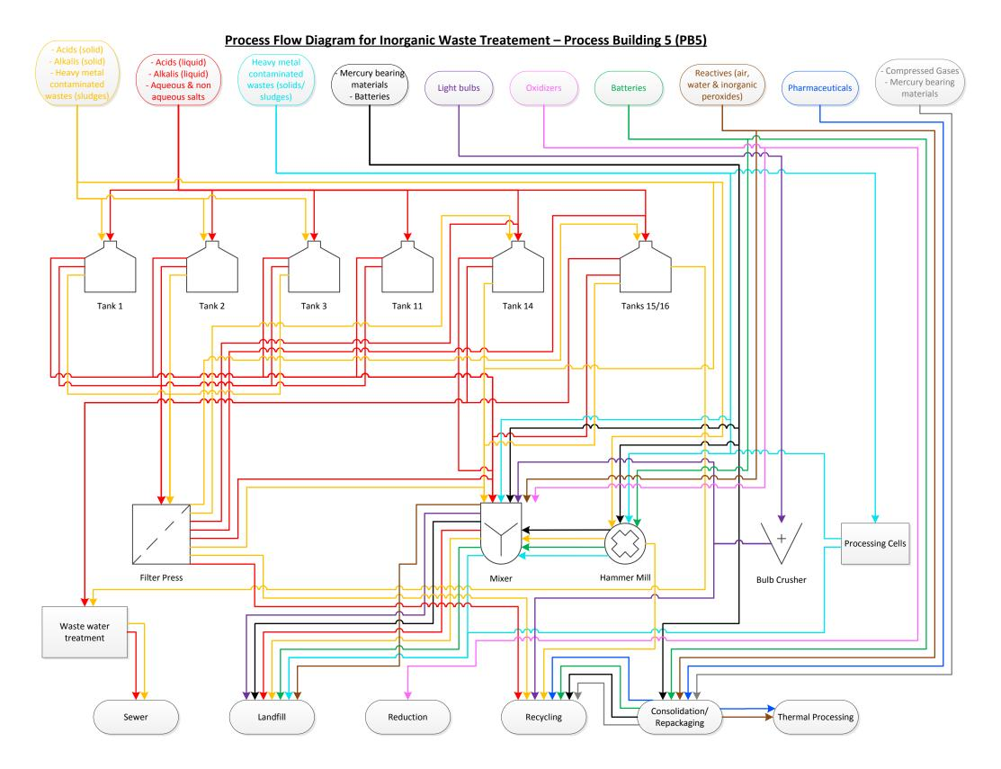
Process Flow Diagram for Inorganic Waste Treatement – Process Building 5 (PB5)
