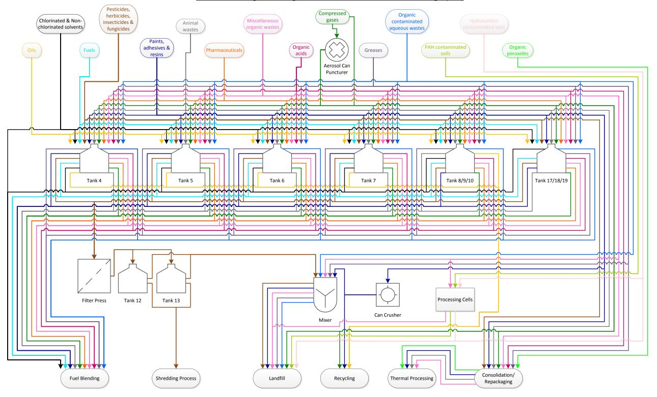
Process Flow Diagram for Organic Waste Treatement – Process Building 1 (PB1)
