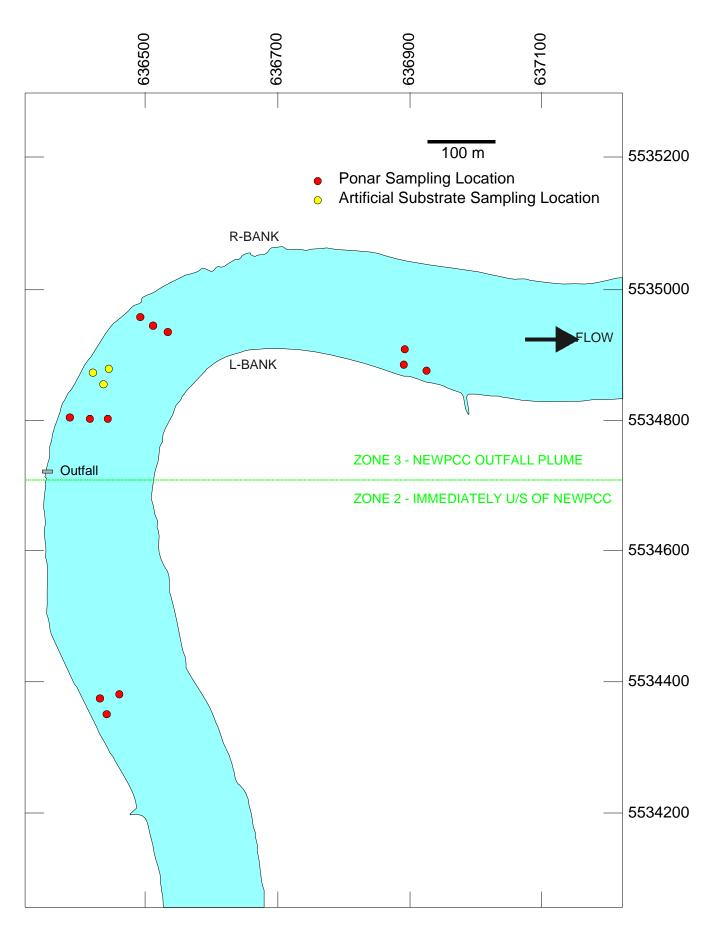
Figure 5. Ponar and artificial substrate sampling locations immediately upstream and downstream of the NEWPCC outfall, September, 1999 (grid in UTMs).
