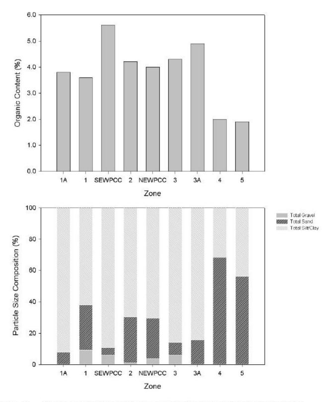
Figure 13. Organic content and particle size composition of sediments collected in Ponar dredge samples in the Red and Assiniboine rivers, September, 1999.
