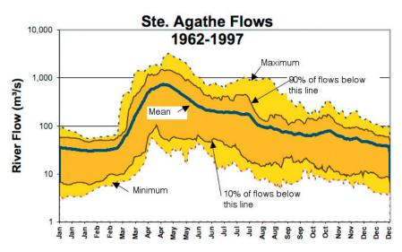
Figure 5: Measured river flows plotted for the Red River at St. Agathe from 1962 to 1999. Flows in the Rivers are extremely variable.
