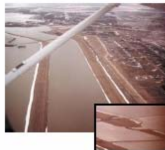
During the 1997 Flood, the existing Floodway Channel was operated at 95% of its safe discharge capacity. A similar flood with high rains would present capacity problems for the existing channel design.
