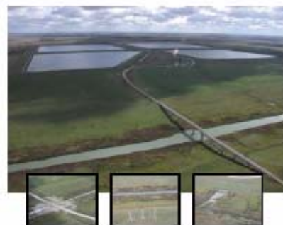
The Floodway Channel is crossed by bridges (top), roads, hydro transmission lines, drainage structures and other crossings. All of these crossings require modification.
