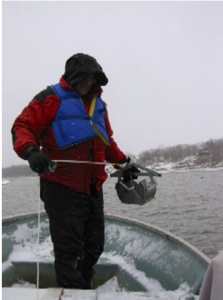
Photograph 6: Ponar sampler used to sample bottom substrate in the Red River in the vicinity of the Floodway Outlet
