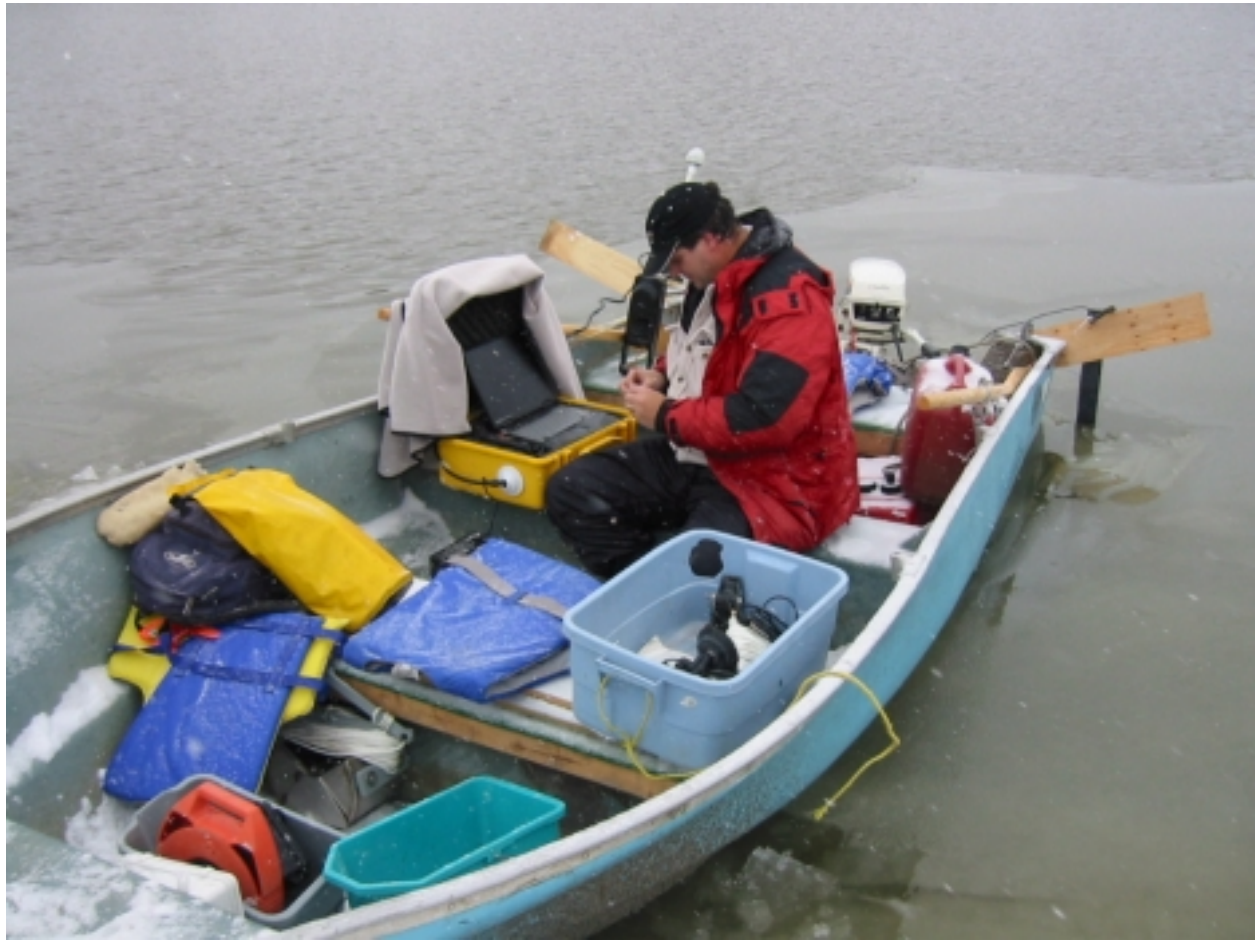
Photograph 5: Recording bathymetry of the Red River in the vicinity of the Floodway Outlet using a PCSounder® (a GPS-linked bathymetry sounder).
