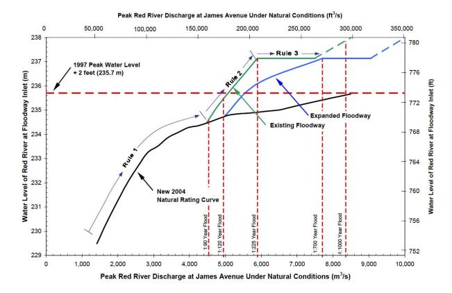
Figure 6 – Rule Curve for Existing and Expanded Floodway
