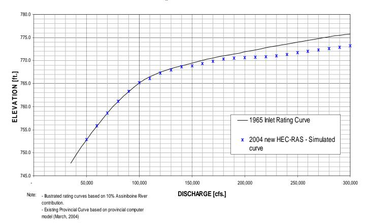
Figure 4: Rating Curve at Inlet Control Structure
