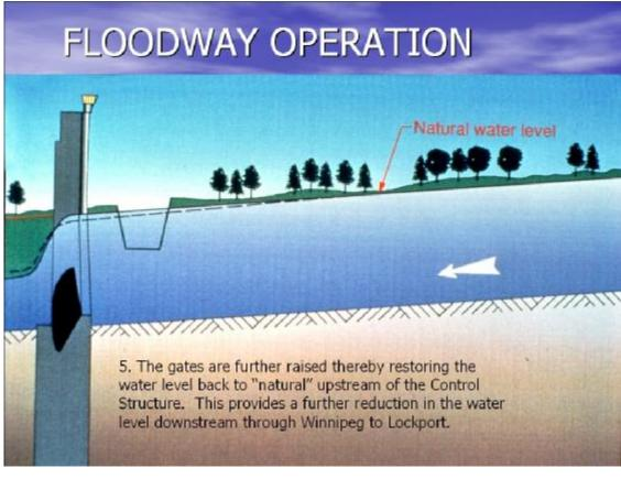
The above graphics demonstrate the gate operation for a given natural flow of approximately 60,000 cfs in the Red River, upstream of the Inlet Control Structure.
