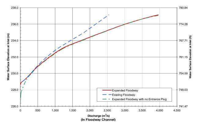
Figure 5 – Rating Curves of Floodway Channel at Floodway Entrance
