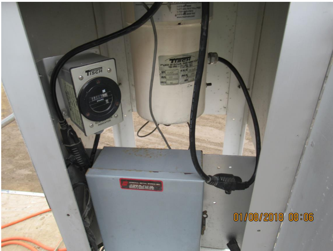
Industrial Metals, Winnipeg, MB, July/August 2018 AMBIENT AIR QUALITY AND ASSESSMENT Photograph 5: Interior of Hi-Vol Sampler Tisch TE-5170
