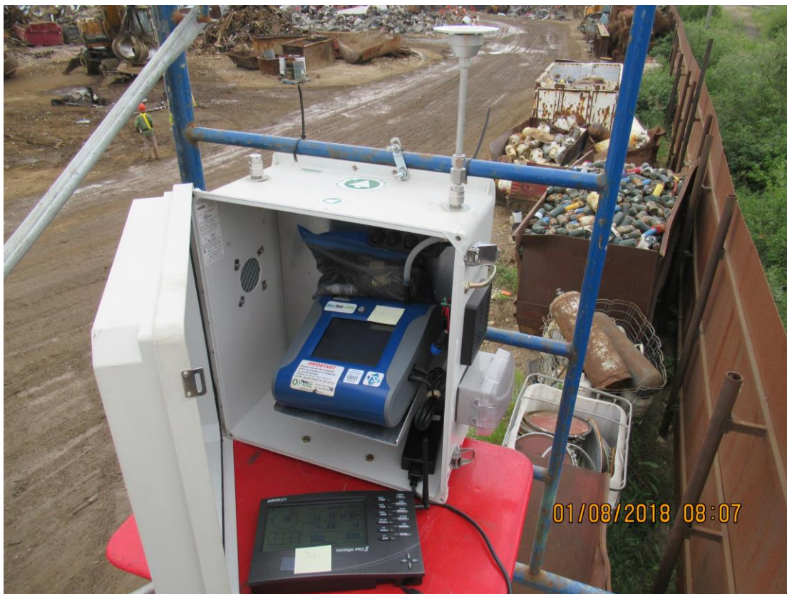
Industrial Metals, Winnipeg, MB, July/August 2018 AMBIENT AIR QUALITY AND ASSESSMENT Photograph 6: PM Monitor Dust Trak DRX and Weather Station Console Vantage Pro 2 at Air Sampling Location IM-1
