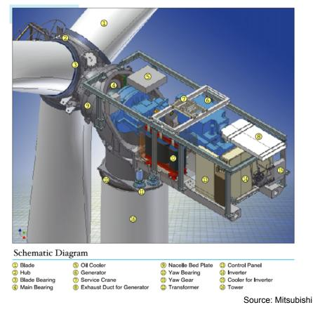
Figure 2-4: Example of Nacelle Components
