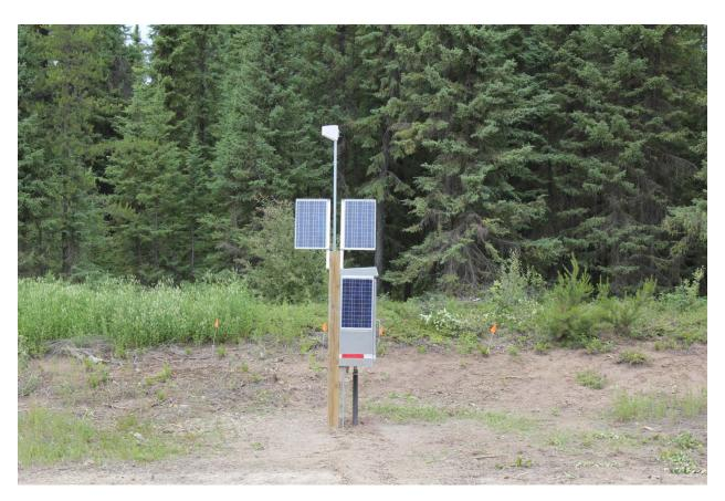
Figure 4-1 Traffic monitoring station
