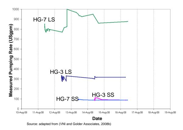
Figure 7.6-8 Pumping Rates during the August 2008 Pump Test
