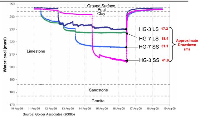
Figure 7.6-7 Water Levels during the August 2008 Pump Test
