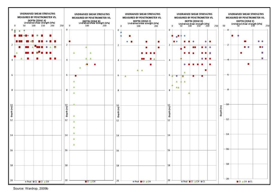
Figure 7.3-6 Variation of Undrained Shear Strengths of the Clay with Depth by Zones
