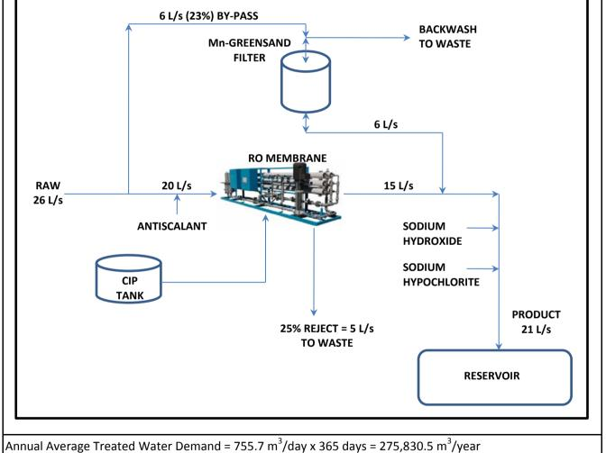
(5 L/s Reject) / (21 L/s Product) x 100 = 23.8 % Reject per unit of water produced
