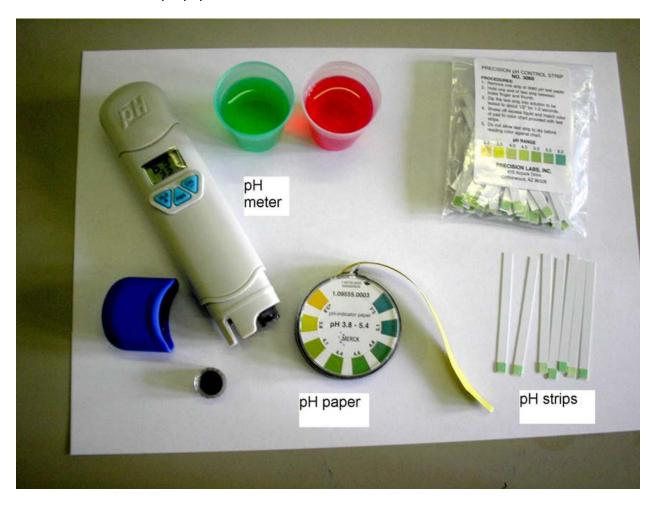
Ensure that the pH test is conducted on the acidified rice once the vinegar mixture has been evenly distributed to assure a target pH of 4.6. If using a probe pH meter, ensure proper calibration by following manufacturer's instructions.
