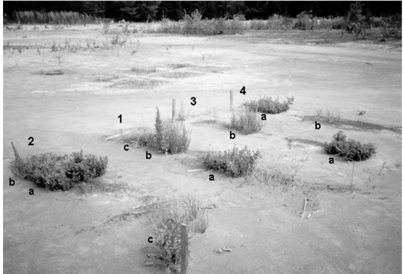
Figure GS-24-3: Site 4, three months after seeding. (area 1 is the control area (0 g/kg C); area 2 had 2 g/kg C applied; area 3 had 3 g/kg C applied; area 4 had 4 g/kg C applied; a is alfalfa; b is slender wheatgrass; c is meadow fescue).
