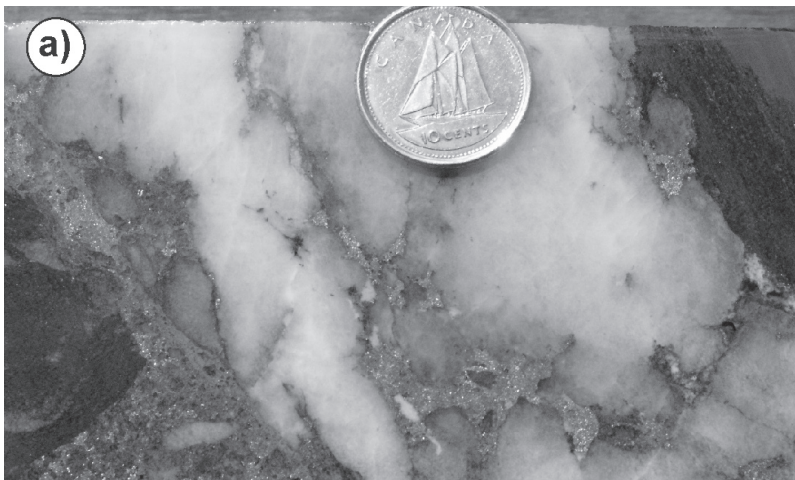
Figure GS-2-4: Base-metal–associated gold mineralization: a) mineralized quartz vein from split drillcore, showing white vein quartz, light grey sulphide (mainly chalcocopyrite and sphalerite) and a lens of dark grey, biotite-altered wallrock; sulphides are located along fractures in the quartz vein or along the margins of the vein; b) north end of the North Star drift, looking up at the back, with north toward the top of the picture; white material is quartz vein, which forms the main mineralized quartz vein in the North Star deposit, and dark material is sheared mafic hostrock; ellipse highlights sulphides, which are mainly located on the east side of the vein.
