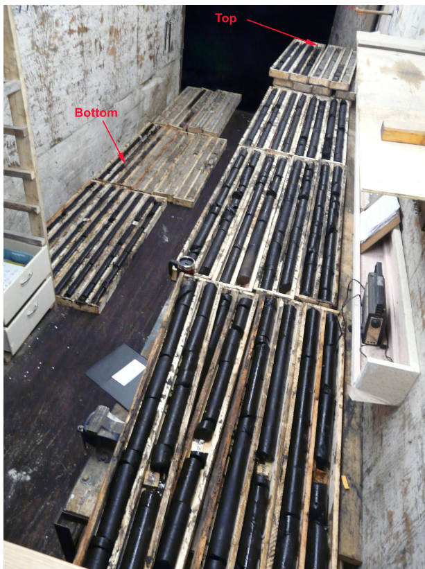
Figure GS-15-4: A 46 m intercept of continuous coal. Each box is 1.5 m long.
