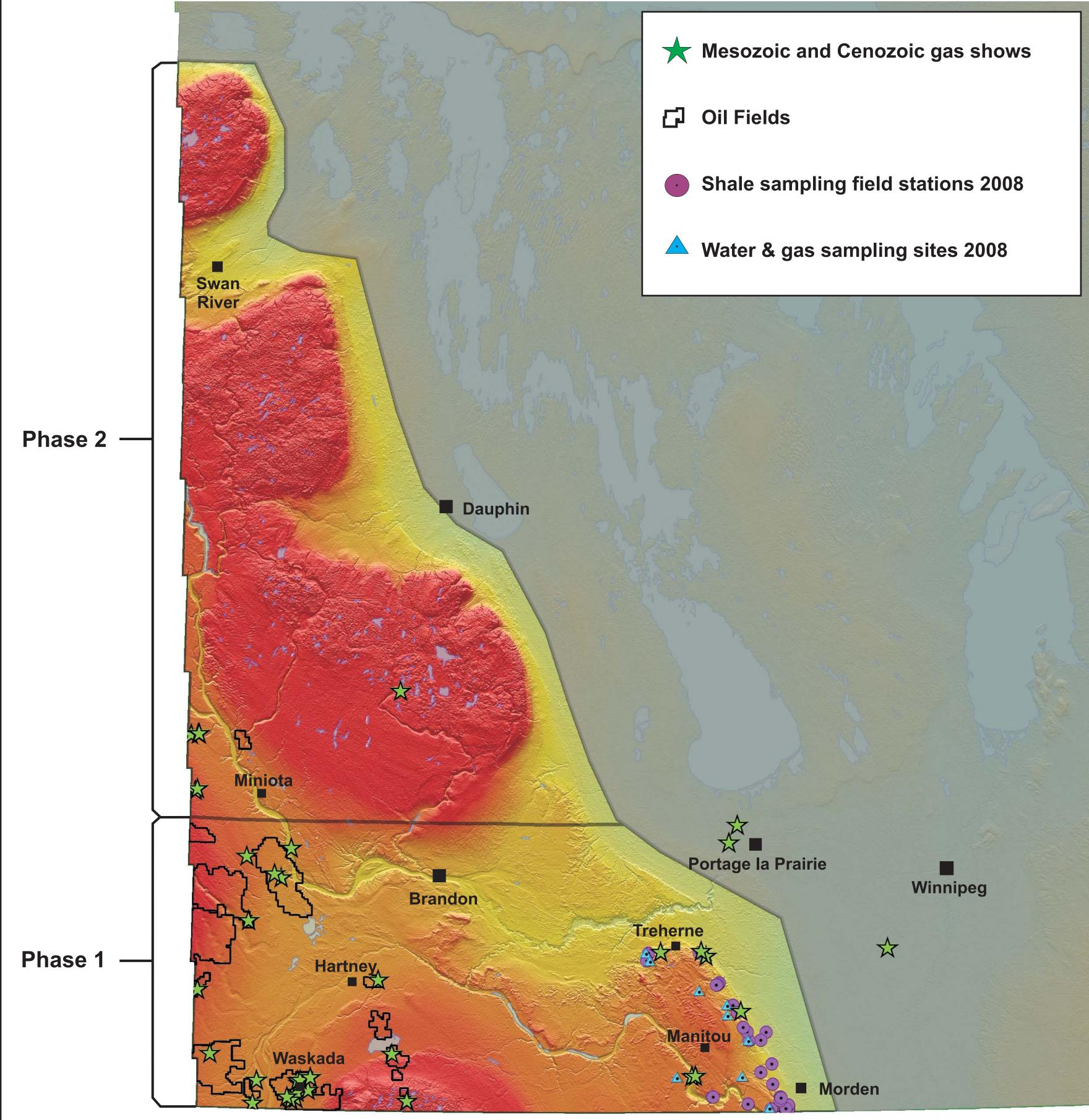
Figure 2: Digital elevation model showing the study area of the Shallow Unconventional Shale Gas Prospects Project, the location of Phase 1 and Phase 2 of the project, Mesozoic and Cenozoic gas shows in relation to extisting oil fields, field station and water/gas sampling sites of the 2008 sampling program.
