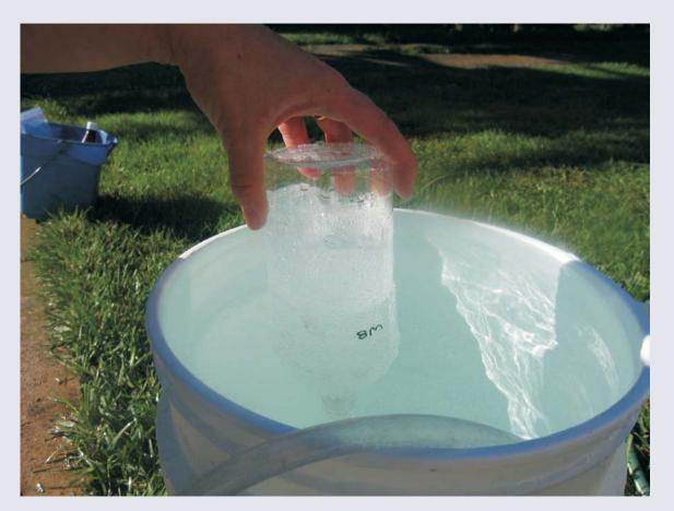
Collection of effervescent water sample; note gas bubbles in water and gas-filled head space in bottle.
