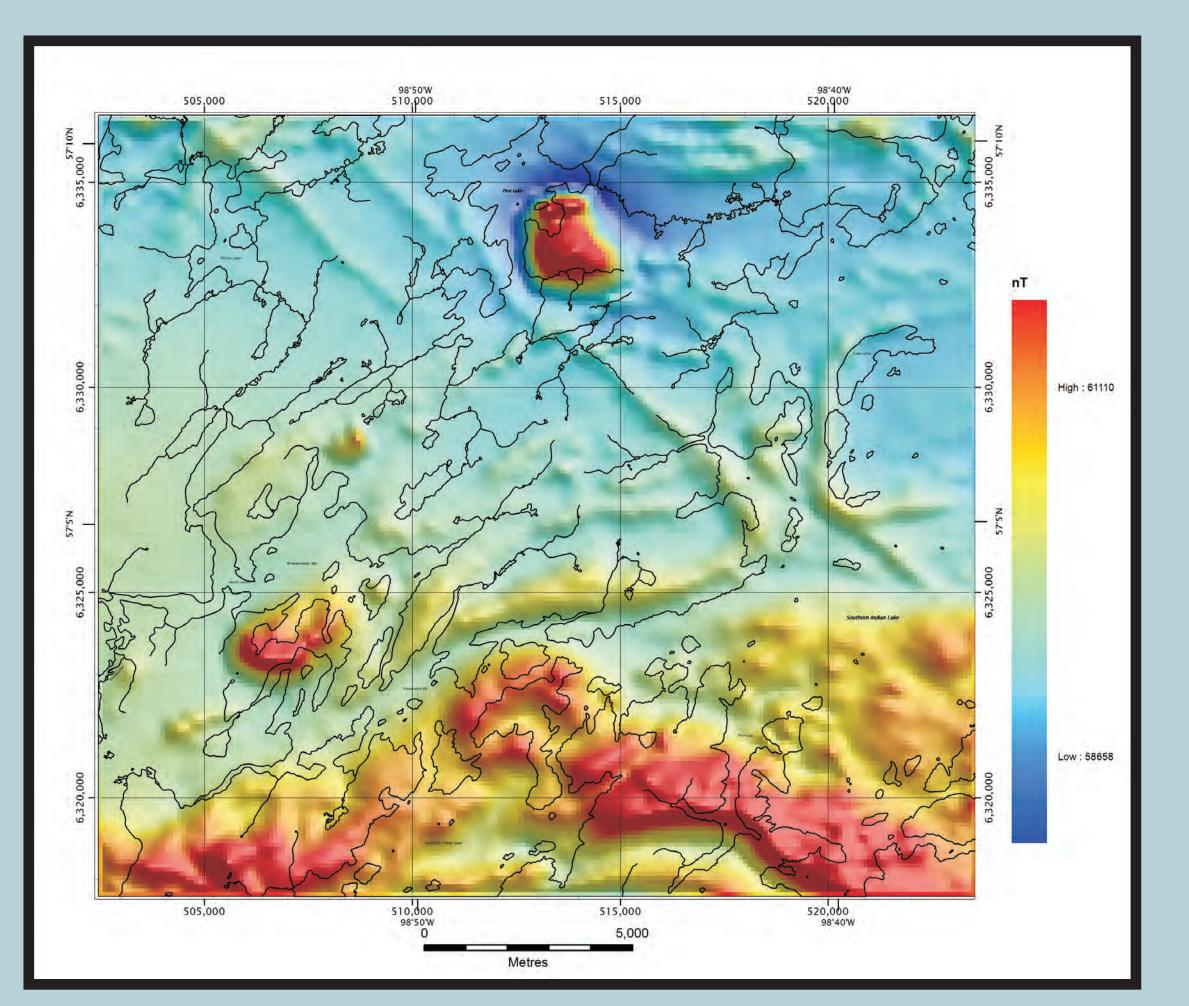
Figure 2. Part of the aeromagnetic survey showing total magnetic intensity of the area depicted in Figure 3. The survey was flown at 300 metre line spacing in the spring of 2008 by the Geological Survey of Canada.
