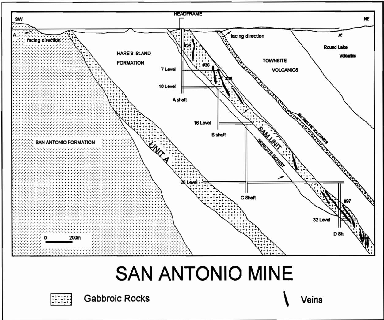
Figure 36: Geological cross-section through the San Antonio Mine.
