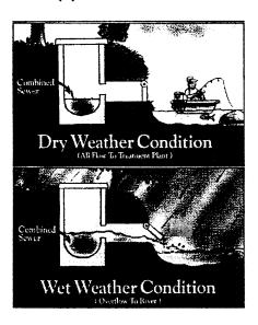
During wet weather the combined volume of wastewater and stormwater runoff is often greater than the capacity of the system. The excess flow is discharged directly to the river at various overflow points in the sewer system. During dry weather, combined sewer systems carry all the wastewater to treatment plants.
