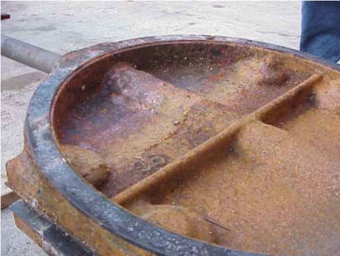
Valve plate and guide channel of side of valve.
