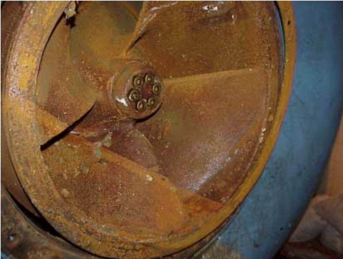
Lower photo of pump impeller - photo shows no damage to impeller.
