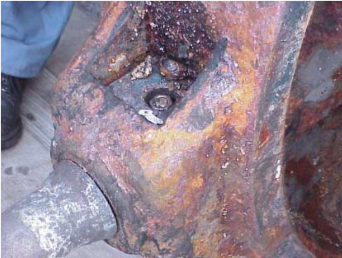
Valve stem attached to valve plate and connecting pins in place.
