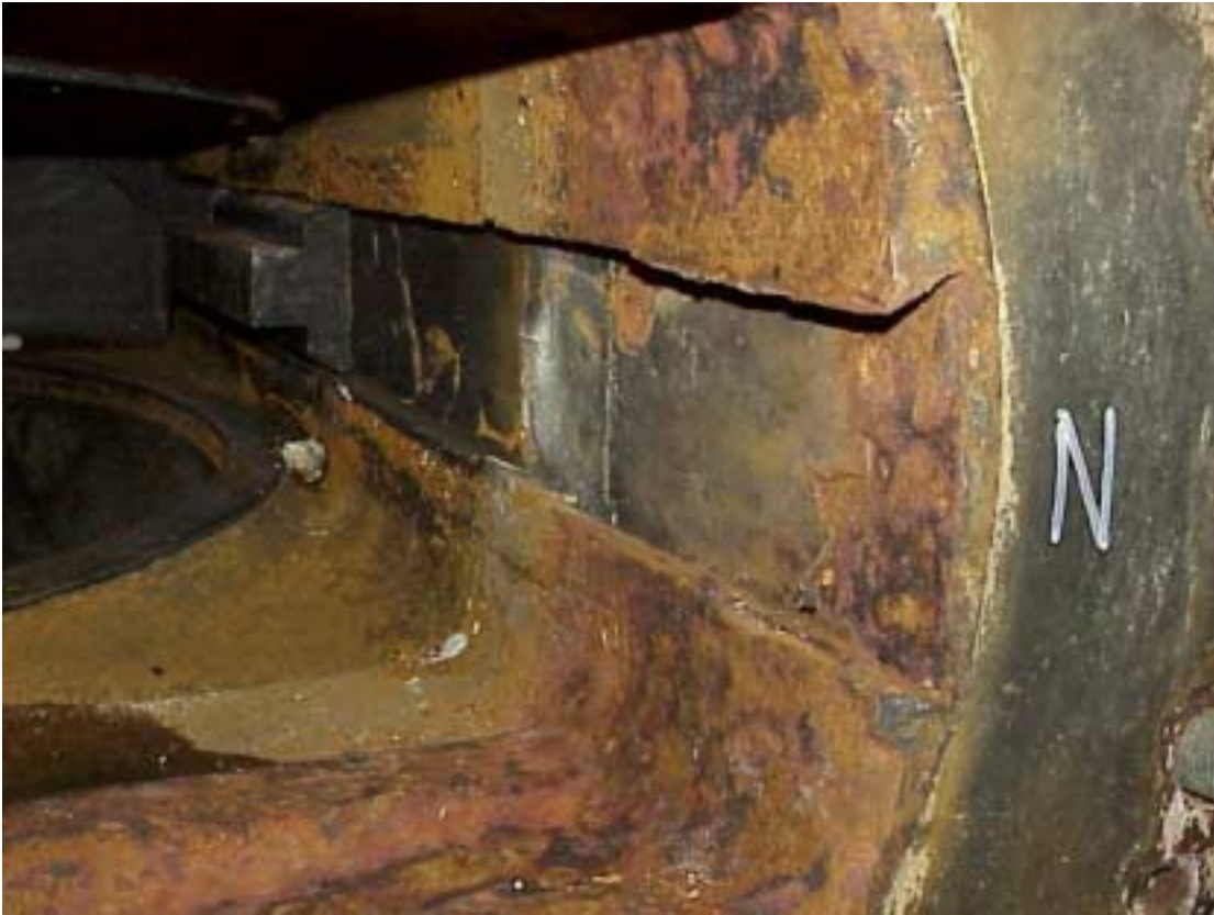
Photo of lower valve body - guide bar from the bonnet is shown located in the lower portion of the valve body.
