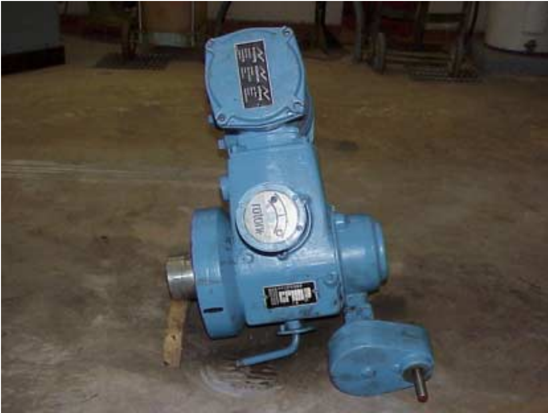
Photo shows Rotork actuator - manual crank wheel would be attached to right side of the unit.
