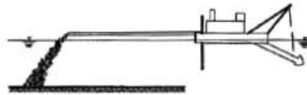
Surface Discharge with Pipeline
