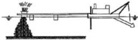
Spreading with Pipeline and Baffle Plate or Box
