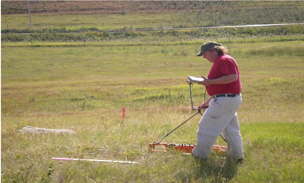
FIGURE 1 GEOPHYSICAL SURVEYING USING AN EM 38 ELECTROMAGNETIC GROUND CONDUCTIVITY METER AND DATA LOGGER.
