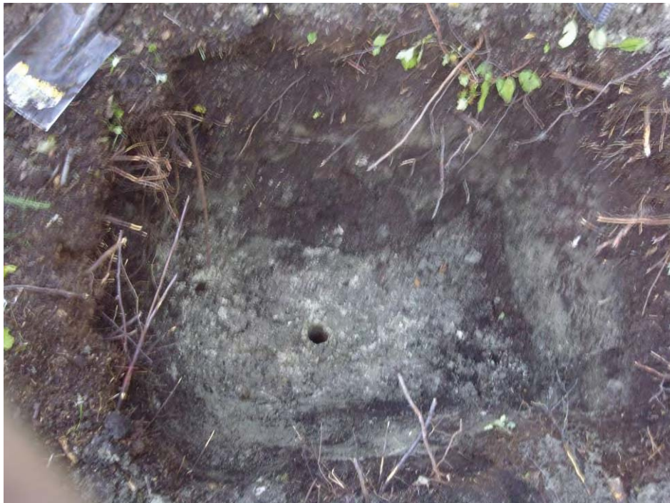
Photo 4 – Auger hole at base of testpit
