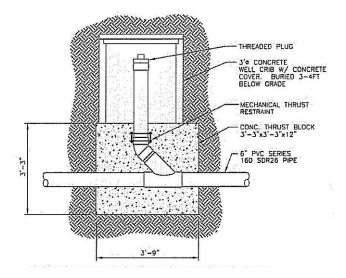
**4.10.** Thrust Blocks – The design and installation of thrust blocks shall be completed according to WAS Design Guidelines for Water and Sewer Section 5.2. Concrete thrust blocks shall be installed at all cleanouts, crosses, tees, elbows, reducers, caps, and inlets, in accordance with the following:
