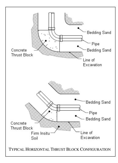
**4.10.1.** The required minimum area, in square metres (m<sup>2</sup>), that a concrete thrust block must bear against undisturbed soil shall be calculated by first dividing the total thrust by the allowable bearing capacity of the soil and then multiplying the result by a safety factor of 1.5, in accordance with the following formula:
