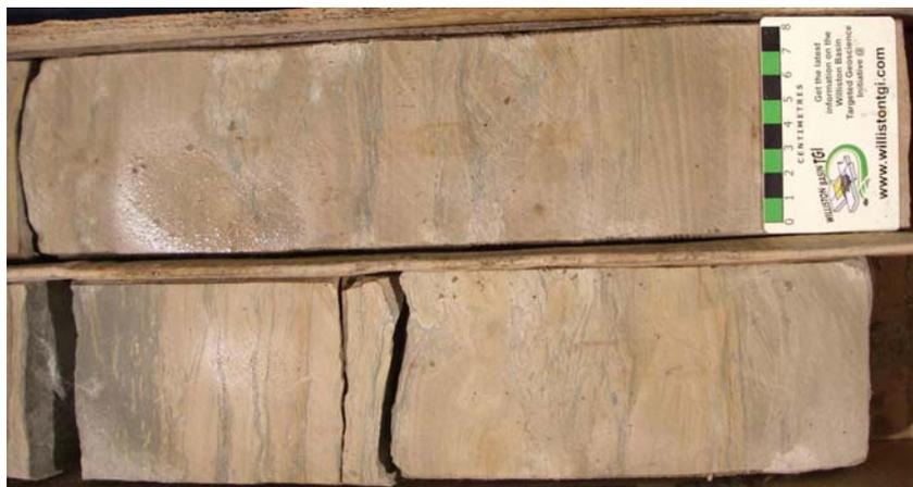
**Figure 5:** Characteristic appearance of subunit 2c in core from 2-8-8-29W1 at a depth of 1003m.
