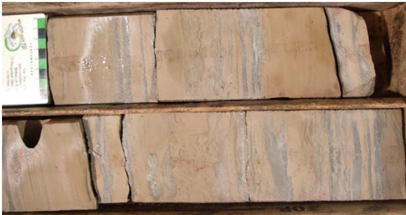
**Figure 9:** Characteristic appearance of subunit 4c in core from 2-8-8-29W1 at a depth of 995m, part of the primary reservoir at Sinclair Field.
