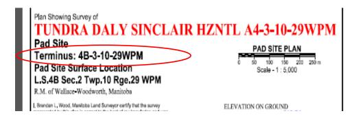
Always refer to the Terminus for the bottomhole Quadrant on the Survey. In this example, the Survey Platte reads:
