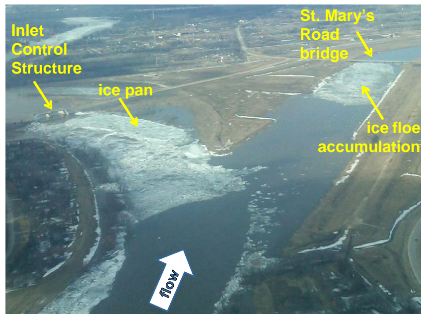
Figure 1: Ice conditions in the area of the floodway inlet on April 7 th , 2011.
