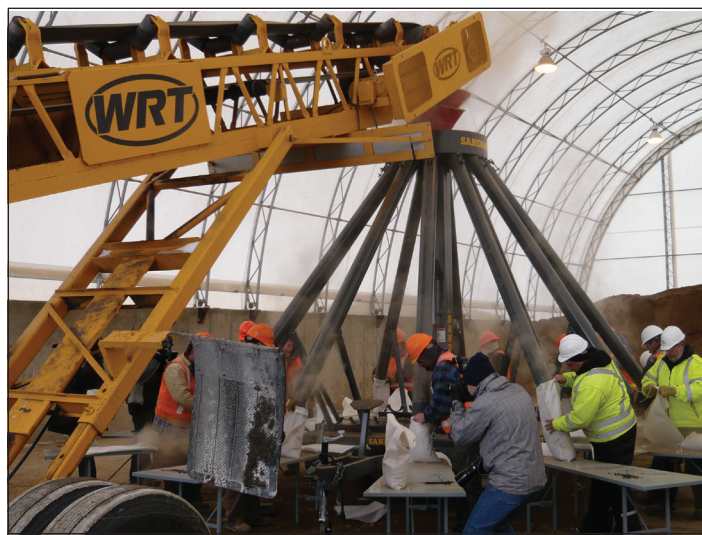
Sandbag filling machine operating in Brandon.
