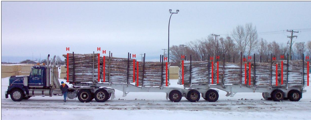
Figure 13 Height measurements taken on a loaded truck
