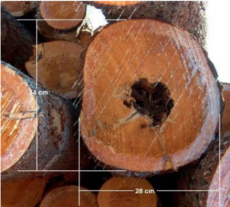
Figure 3 Measuring diameters: logs with irregular sawn surfaces
