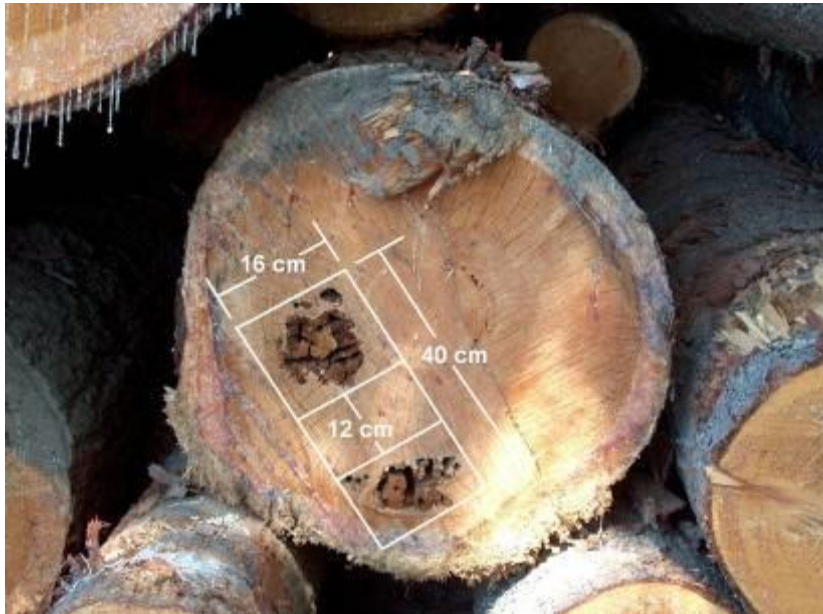
Figure 25 Two defects separated by 14 cm or less
