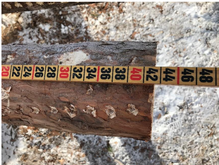
Figure 5 Length class determination in 2 cm class
