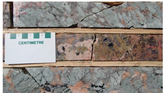
Figure 2: Drillcore from the Zoro Lithium property at Wekusko Lake, showing light green, bladed spodumene (lithium-aluminum-silicate).
