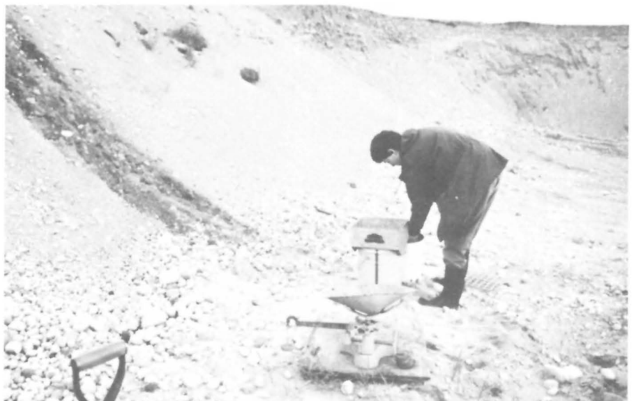
Figure AR-1-2: Equipment including scale and sieves utilized in coarse aggregate field sieving.
