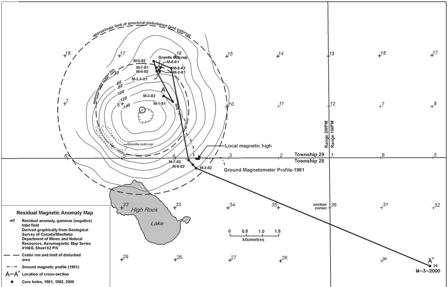
Figure GS-31-2: Location of coreholes in the High Rock Lake structure magnetic map and of cross-section A-A' (after McCabe, 1982).
