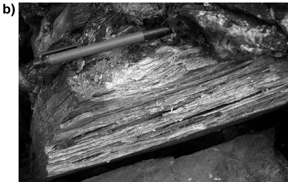
Figure GS-11-4: Felsic phyllonites from the D_2 NSLSZ north of Stear Lake: a) weakly altered felsic phyllonite from the footwall of the shear zone, with alteration characterized by the synshear growth of garnet (g) and magnetite (mt); b) intensely sheared and sericitized pyritic phyllonite from a more central portion of the shear zone.
