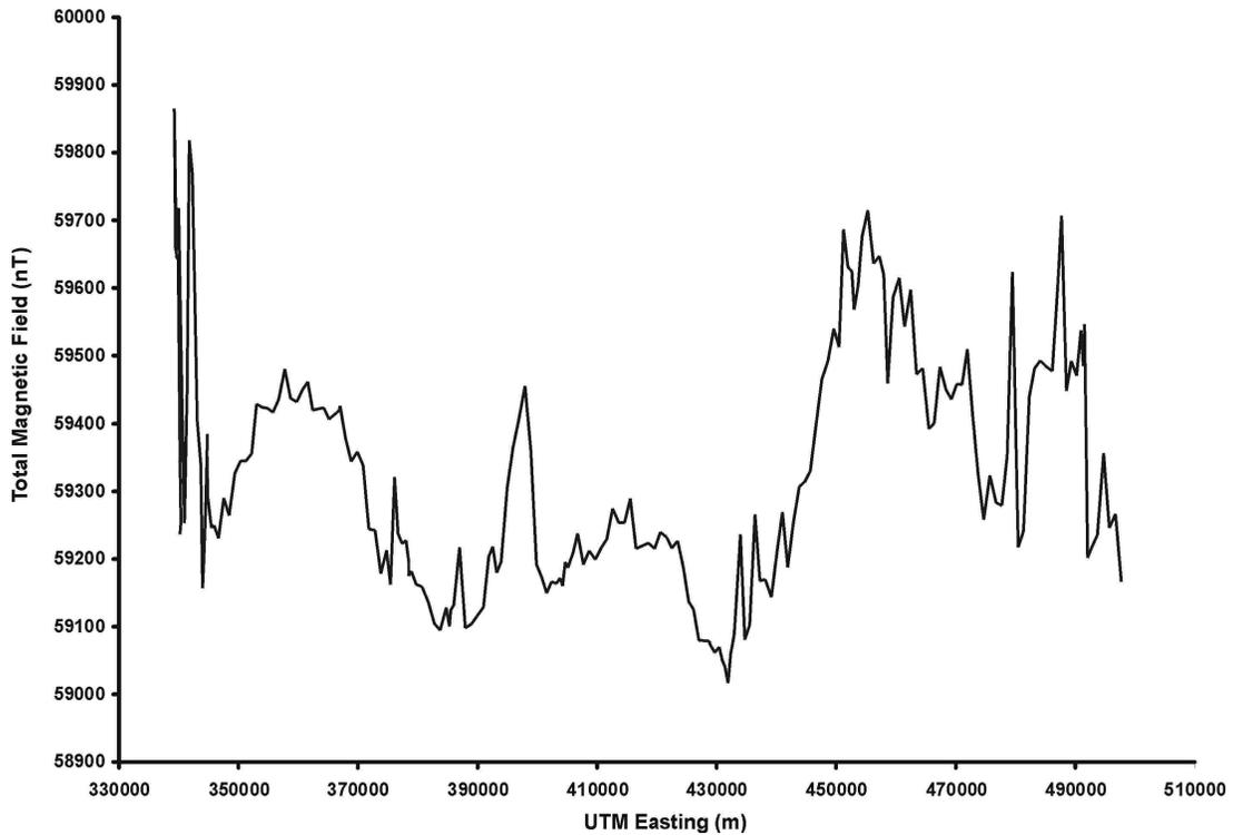
Figure GS-26-6: Profile of total magnetic field response. An inverse relation with the Bouguer gravity anomaly is evident.
