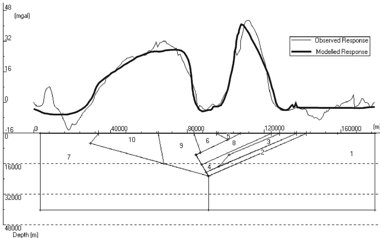
Figure GS-26-5: Preliminary model fitted to the gravity data. The model consists of 10 crustal bodies.
