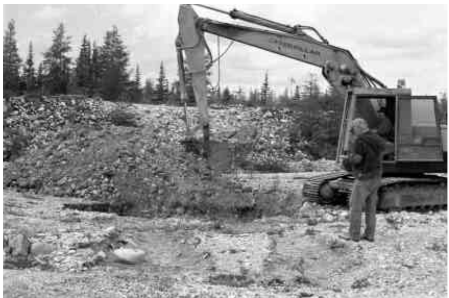
Figure GS-27-2: Backhoe testing at the base of old pit; Twin Lakes deposit.
