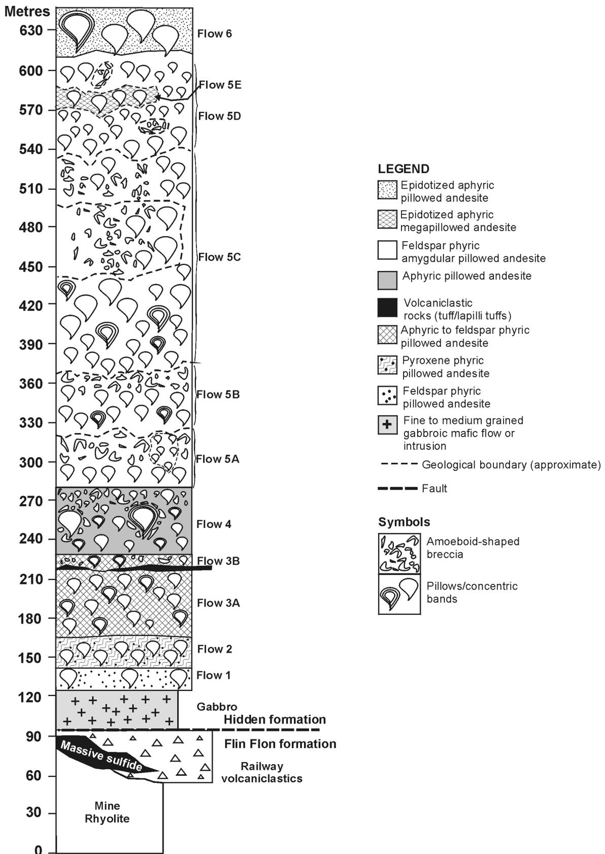
Figure GS-2-4: Stratigraphic section through the Hidden formation above the 777 VMS deposit, based on 1:1000-scale mapping by Tardif (see Figure GS-2-1 for location).
