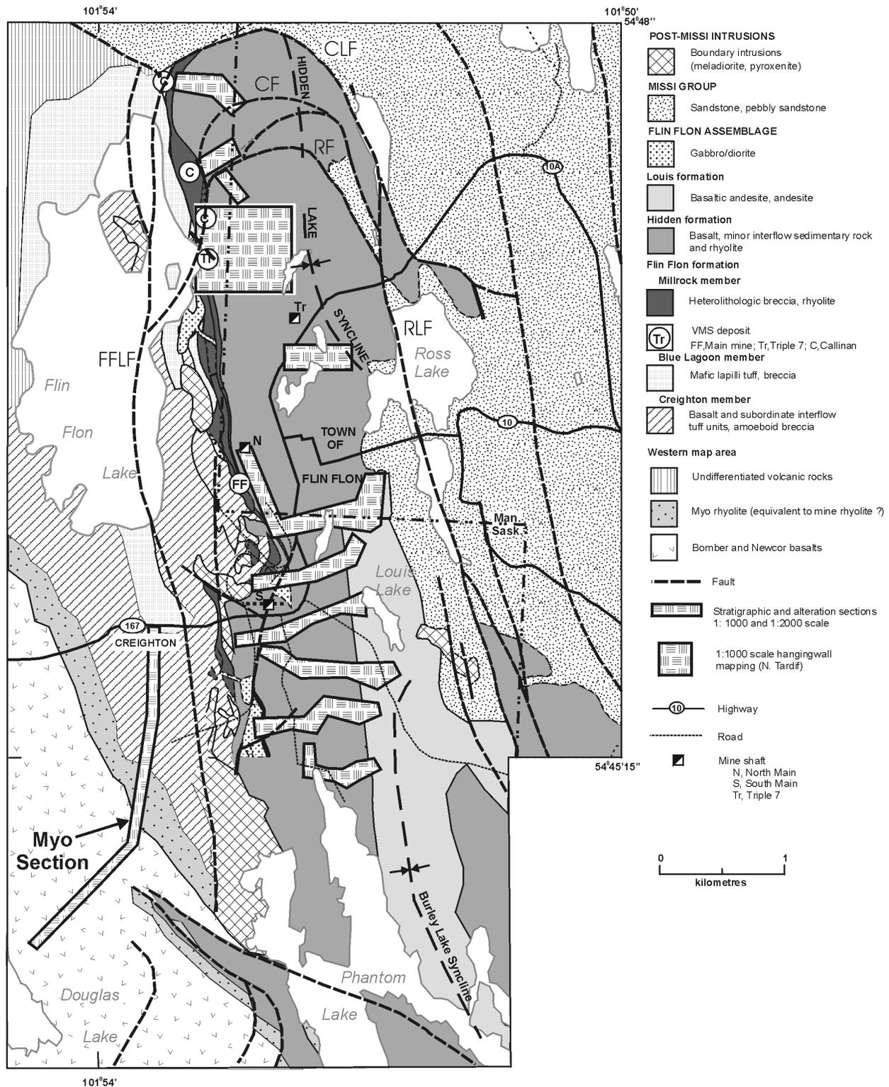
Figure GS-2-1: Simplified geology of the Flin Flon block, showing the location of detailed traverses in the hanging wall of the Flin Flon-777-Callinan VMS horizon. Abbreviations: CLF, Club Lake Fault; CF, Catharine Fault; FFLF, Flin Flon Lake Fault; RF, Railway Fault; RLF, Ross Lake Fault.
