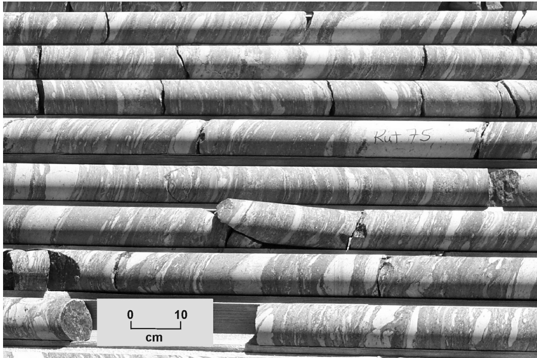
Figure GS-23-3: Angular felsic volcanic fragments in polymictic breccia from drillhole RUT 75. Beds several metres thick are interlayered with possible debris flows.
