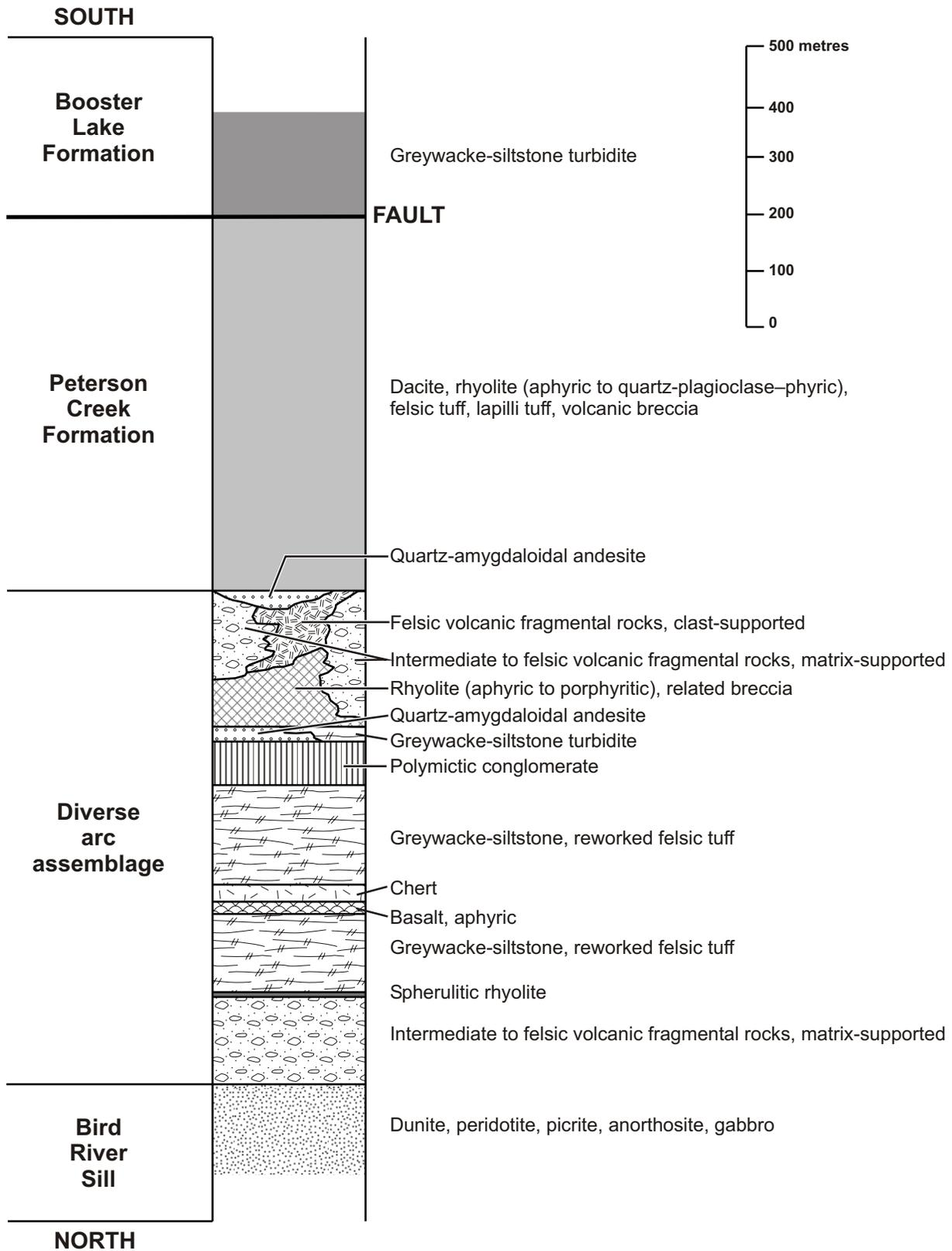
Figure GS-12-5: Stratigraphic column of the Highway Junction section, showing lithostratigraphic details of the diverse arc assemblage, north panel, Bird River Belt.
