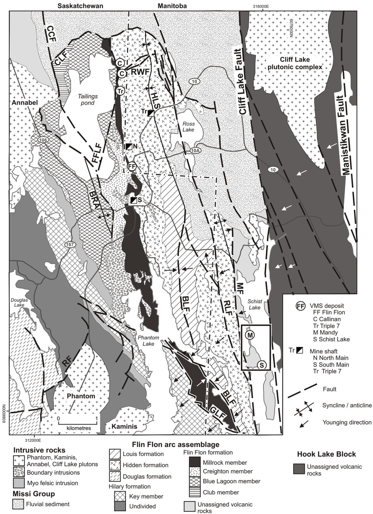
**Figure GS-3-2:** Simplified geology of the Flin Flon area, showing the major structures; box indicates the location of the Schist Lake–Mandy mines area (modified from Simard, 2006). Abbreviations: BLF, Burley Lake Fault; BRA, Beaver Road anticline; CCF, Creighton Creek Fault; CLF, Cliff Lake Fault; FFLF, Flin Flon Lake Fault; GLF, Green Lake Fault; HLS, Hidden Lake syncline; MF, Mandy Road Fault; RF, Rio Fault; RLF, Ross Lake Fault; RWF, Railway Fault.
