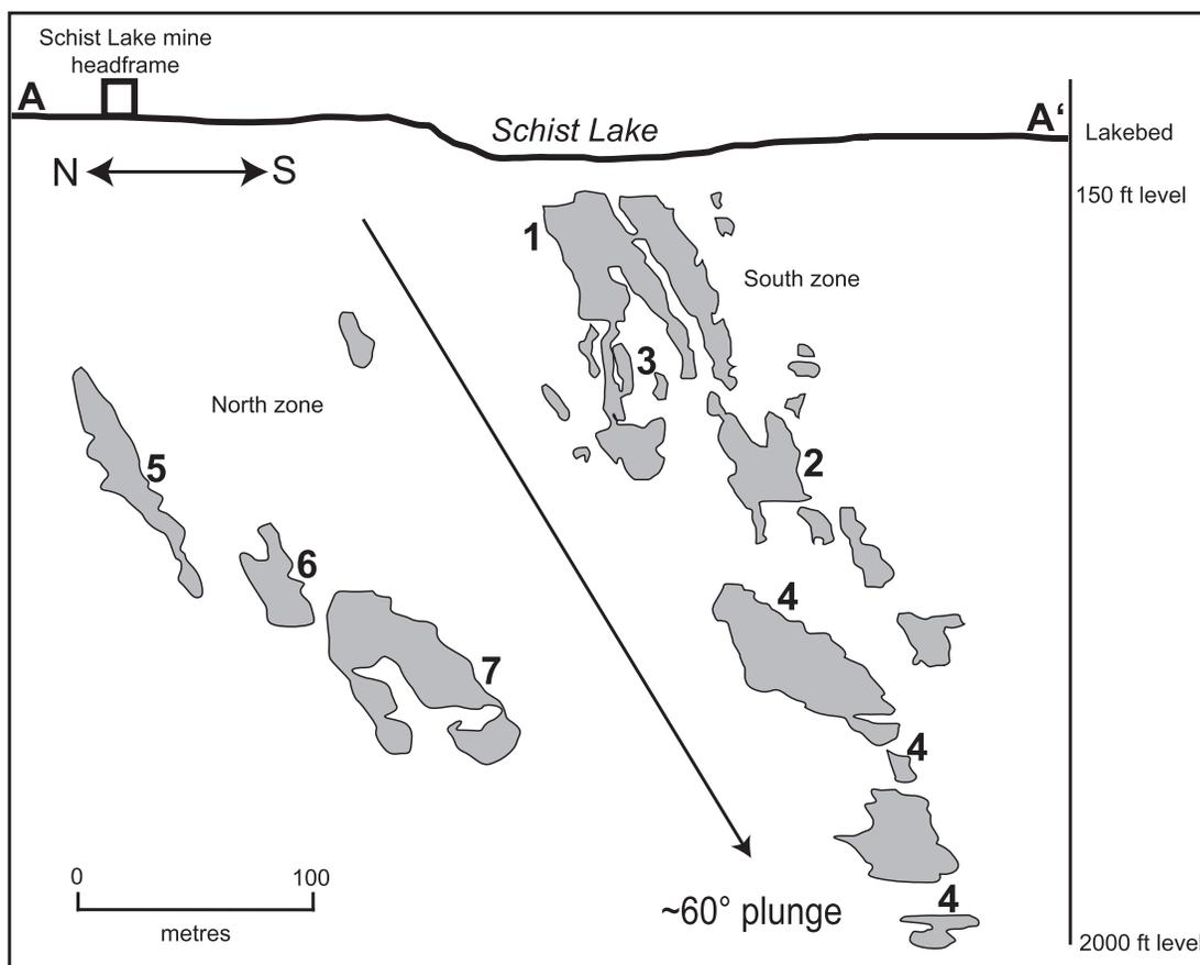
**Figure GS-3-3:** Schematic section of the Schist Lake orebody (from Hudson Bay Exploration and Development Co. Ltd. archive data). Numbers 1–4 represent the ore lenses in the south zone and numbers 5–7 represent the ore lenses in the north zone. See Figure GS-3-4 for location of section.
