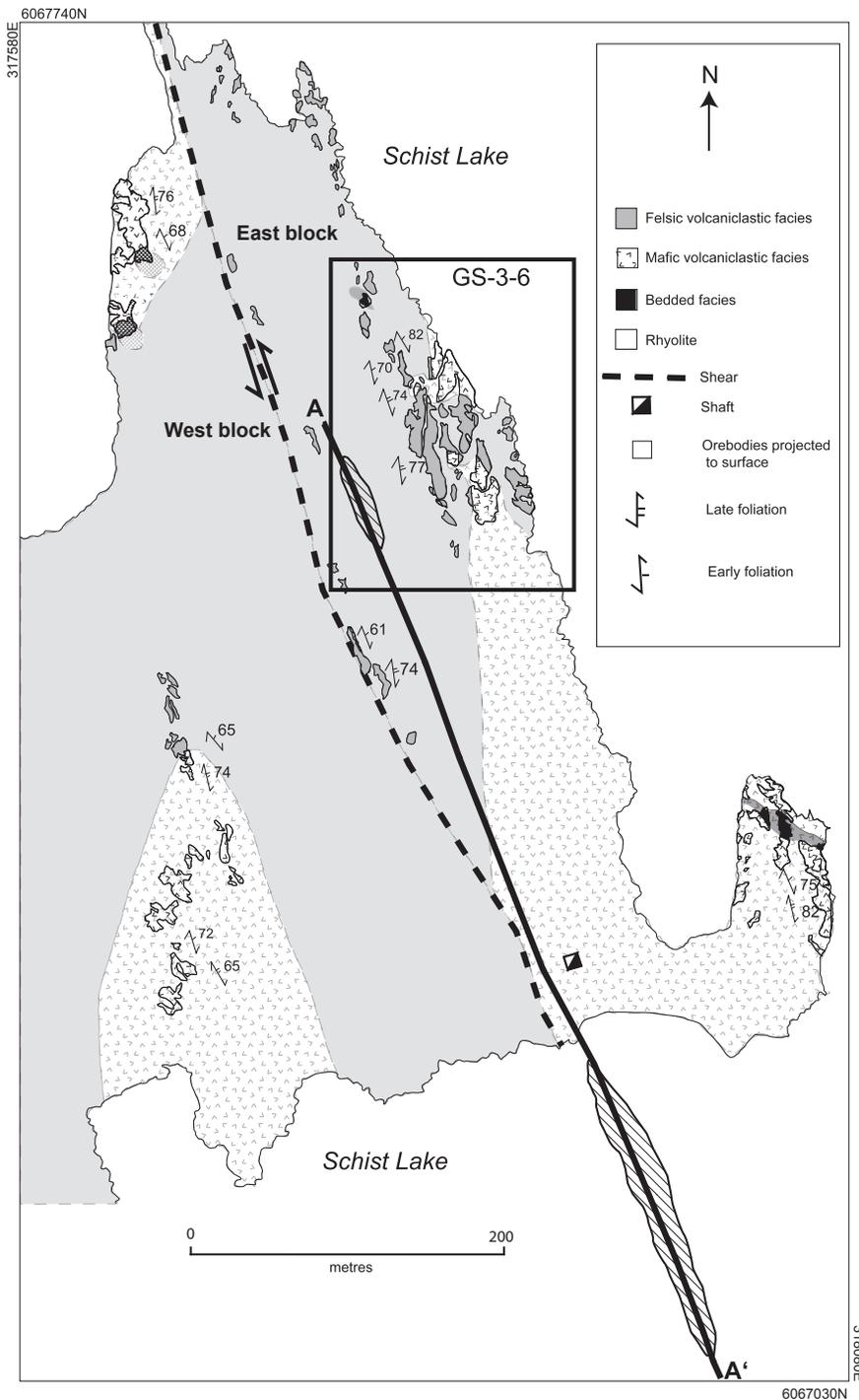
**Figure GS-3-4:** Geology of the Schist Lake mine peninsula, including the surface projection of the orebody and the location of the shaft; box indicates the location of the alteration map (Figure GS-3-6). A–A' represents the line of section in Figure GS-3-3.
