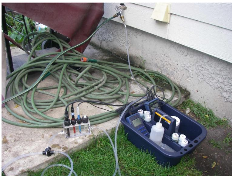
**Figure GS-18-3:** Water sampling set-up showing flow-through cell with probes; photo taken at sampling site in SW-6-6-8-W1.
