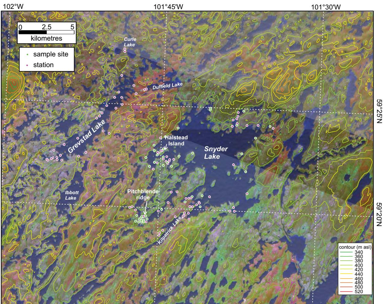
**Figure GS-2-1:** Study area in far northwestern Manitoba with fieldwork based out of camps on Snyder and Grevstad lakes. Sample sites and mapping stations are shown. Background image was generated by draping SPOT 4 imagery over a Shuttle Radar Topography Mission (SRTM) digital elevation model (United States Geological Survey, 2004).
