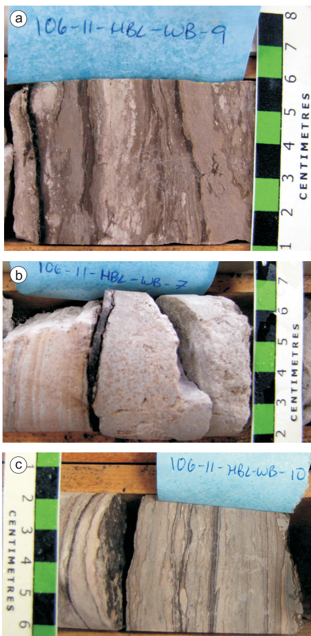
Figure GS-11-4: Core of dark brown laminated oil shale from the Merland et al. Whitebear Creek Prov. well, northeastern Manitoba (see Figure GS-11-1 for location). Oil shale in the Red Head Rapids Formation at depths of a) 220.98 m and b) 221.28 m and in the Severn River Formation at a depth of c) 179.98 m. Scale is in centimetres.
