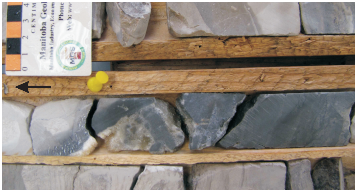
Figure GS-11-7: Core showing potential hydrothermal dolomite in the Severn River Formation in the Houston Oils et al. Comeault Prov. No. 1 well, northeastern Manitoba (see Figure GS-11-1 for location), at a depth of 411.8 m; scale is in centimetres.
