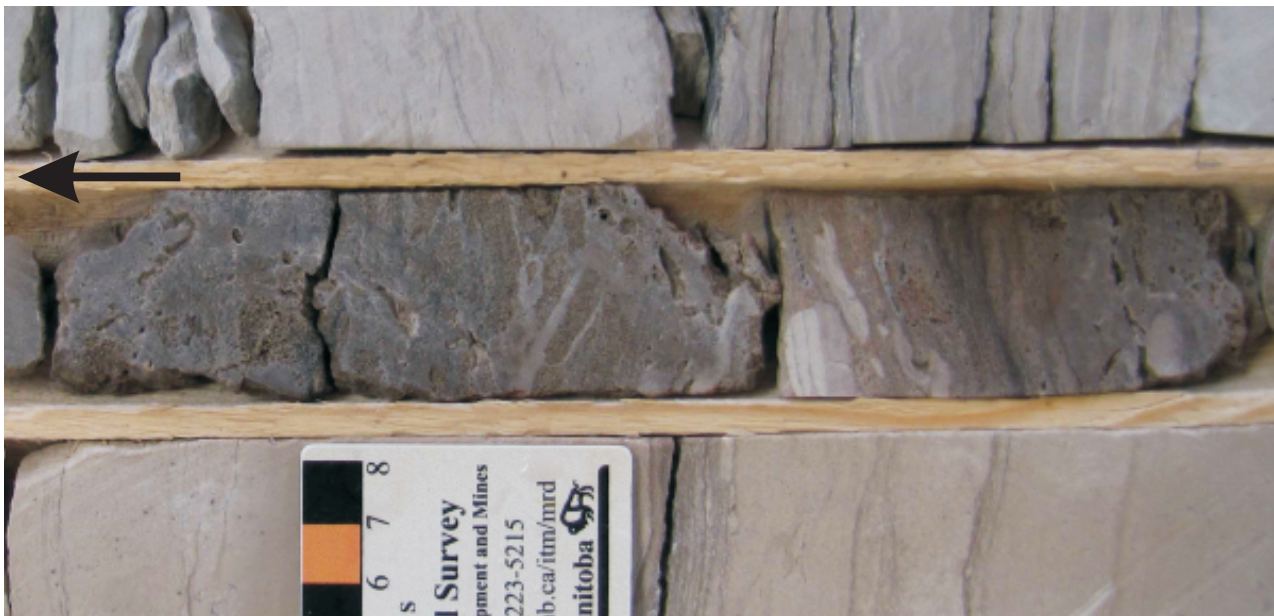
Figure GS-11-3: Core showing potential oil staining of the Severn River Formation in the Houston Oils et al. Comeault Prov. No. 1 well, northeastern Manitoba (see Figure GS-11-1 for location) at a depth of 415.4 m; scale in centimetres.
