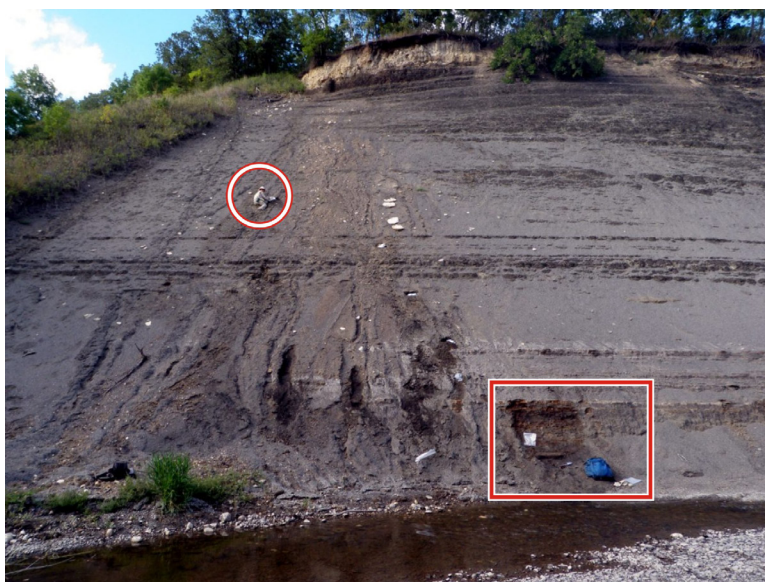
Figure GS-13-5: Gammon Ferruginous Member outcrop in L.S. 15, Sec. 15, Twp. 23, Rge. 20, W 1 st Mer. M. Nicolas (shown within circle) is positioned approximately halfway up the steeply sloping outcrop, above the Pembina Member-Gammon Ferruginous Member contact. Oxidized Gammon Ferruginous Member was sampled from a freshened surface near the base of the outcrop over a 1.25 m interval (shown within square).
