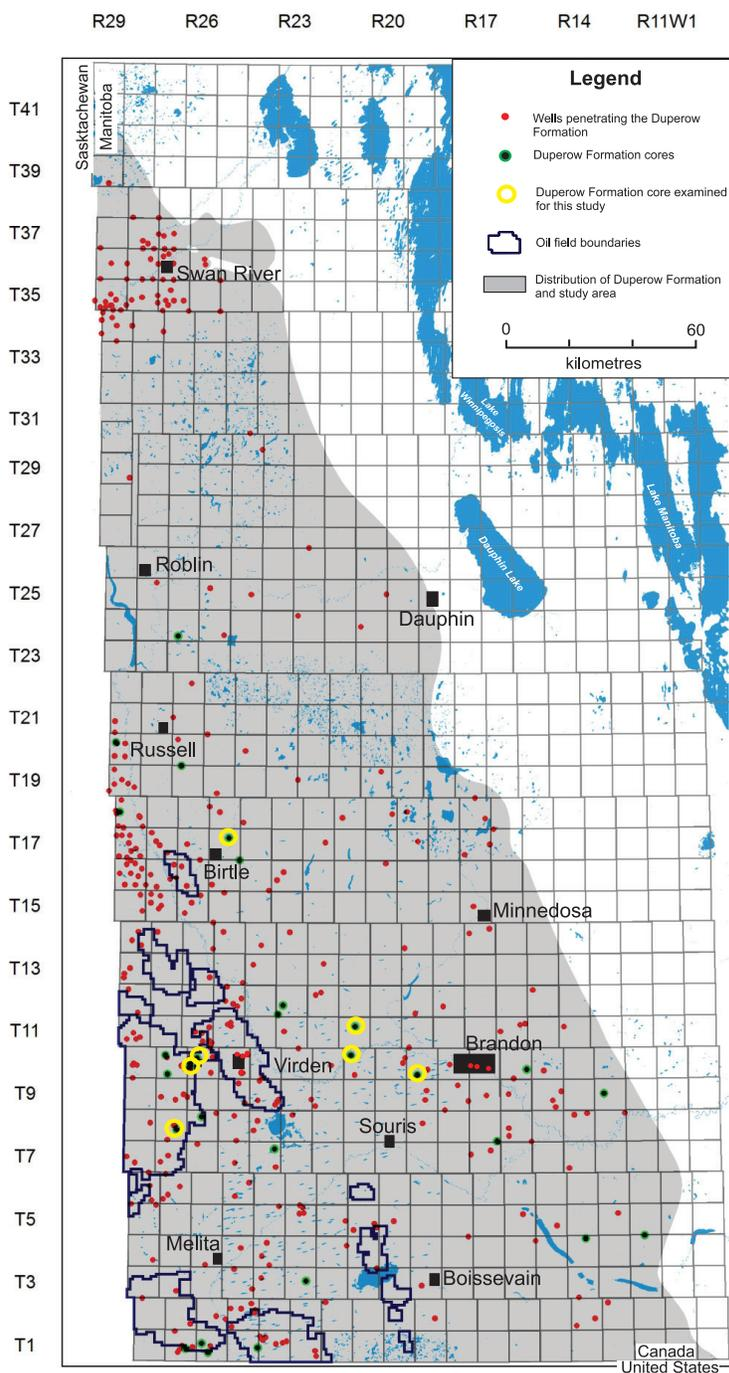
**Figure GS-15-1:** Distribution of the Duperow Formation in southwestern Manitoba, wells that penetrated the formation, wells with cores in southwestern Manitoba and core logged for this study.
