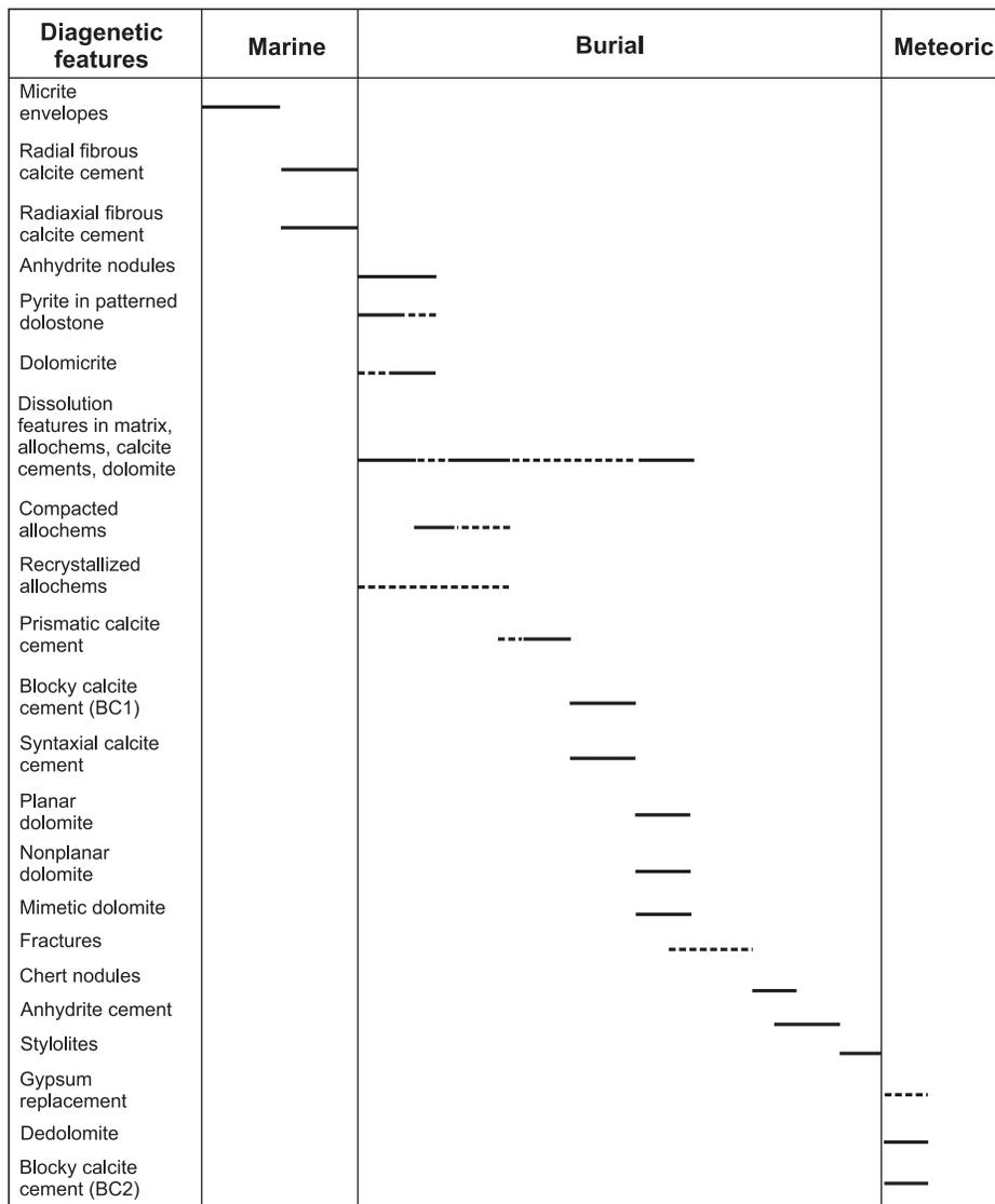
**Figure GS-15-6:** Paragenetic sequence for the Duperow Formation in southwestern Manitoba. The time of formation of each feature is interpreted relative to other described features; the length of the horizontal lines is not an indication of duration (modified from Bates, 2016).
