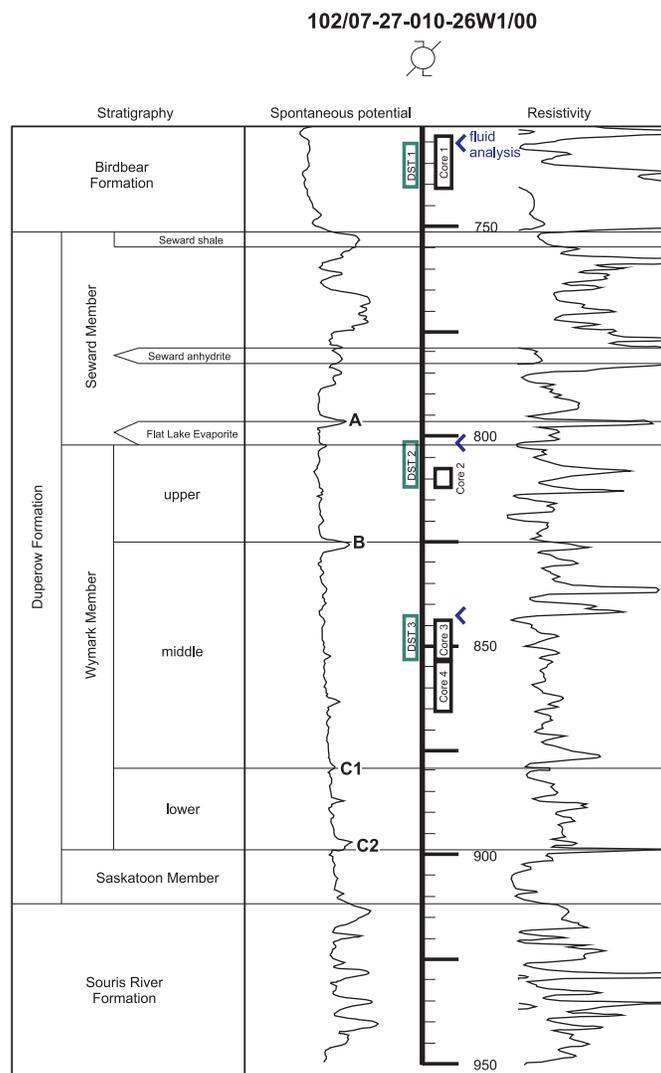
**Figure GS-15-4:** Stratigraphy and typical spontaneous potential and resistivity-log signature of the Duperow Formation from the B.A. Union Grose Virden SWD 7-27-10-26W1 well, southwestern Manitoba. Marker beds defining unit contacts are labelled C3, C1, B and A. Depth is in metres (modified from Egge et al., 2012). Abbreviation: DST, drill stem test.
