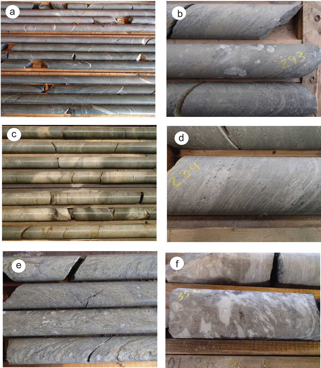
Figure GS-6-4: Photos of drillcore from the Reed Lake area: a) JAS-1; massive andesitic flow with moderate to strong pervasive silica alteration; intervals in photo show a progression from moderate (medium grey-green at bottom) to strong silica alteration (light grey colour at top; BQ core; 68.6–85.3 m [225–280 ft]); b) EEL-313, turbidites of the Burntwood group showing centimetre-thick planar beds of greywacke and mudstone with light grey, randomly-oriented porphyroblasts of andalusite (BQ core; 89.3 m [293 ft]); c) EEL-76, aphyric felsic flow and felsic tuff showing bleached areas that represent zones of moderate to strong pervasive silica alteration (BQ core, 376.1–385.3 m [1234–1264 ft]); d) HP-11-04, quartz-phyric intermediate crystal tuff with moderate sericite alteration (NQ core, 234 m); e) RG-1, quartz-phyric felsic lapilli tuff with weak to moderate sericite alteration (BQ core, 101.5–106.0 m [333–348 ft]); f) SP-12-01, basaltic amoeboid pillow breccia with narrow dark selvages on clasts and a fine matrix of biotite and chlorite (HQ core; 35.6 m). Drillcore diameter: BQ, 36.5 mm; HQ, 63.5 mm; NQ, 47.6 mm.
