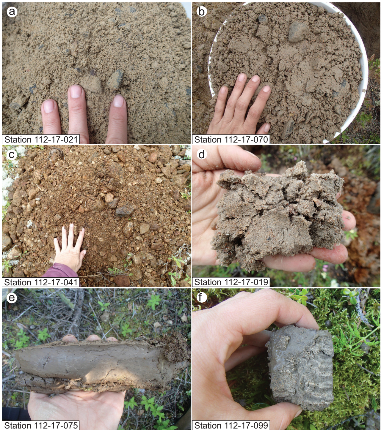
Figure GS2017-17-4: Examples of various sediment types encountered during fieldwork include a) washed till that has a sandy texture, b) unwashed till that has a silty sandy texture, c) poorly sorted beach gravel derived from till, d) moderately sorted fine- to medium-grained sand, e) massive clay sampled by an auger, and f) interbedded silt (dark) and sand (light).
