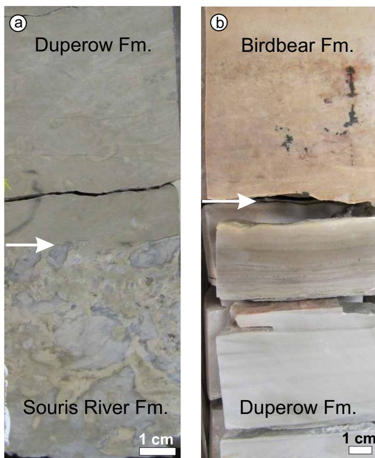
**Figure GS2018-11-4:** Core photograph of lower and upper contacts of the Duperow Formation: **a)** at a depth of 656.26 m between the Souris River and Duperow formations, and **b)** at a depth of 502.90 m between the Birdbear and the Duperow formations, in the Manitoba Potash Corporation (MPC) core at 3-29-20-29W1; arrows mark contacts. Abbreviation: Fm., Formation.
